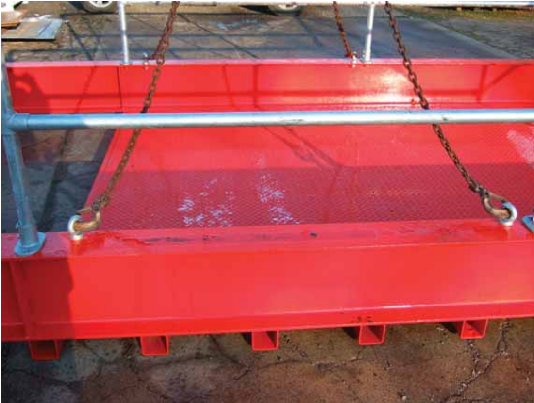
2 ATTATCH CRANE CHAINS TO 4 No LIFTING EYES LOCATED ON THE TOP FLANGE OF THE MAIN BEAMS
