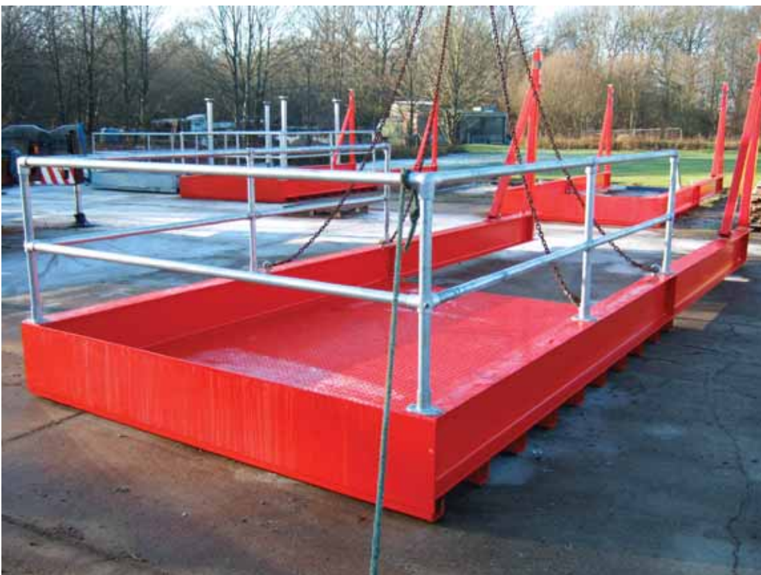
3 ATTATCH TAG LINES TO PLATFORM
